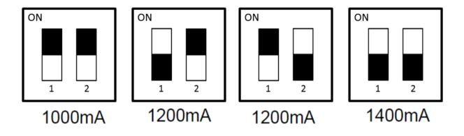
The driver will be shipped out of factory with both switches set to ON (1000mA)
